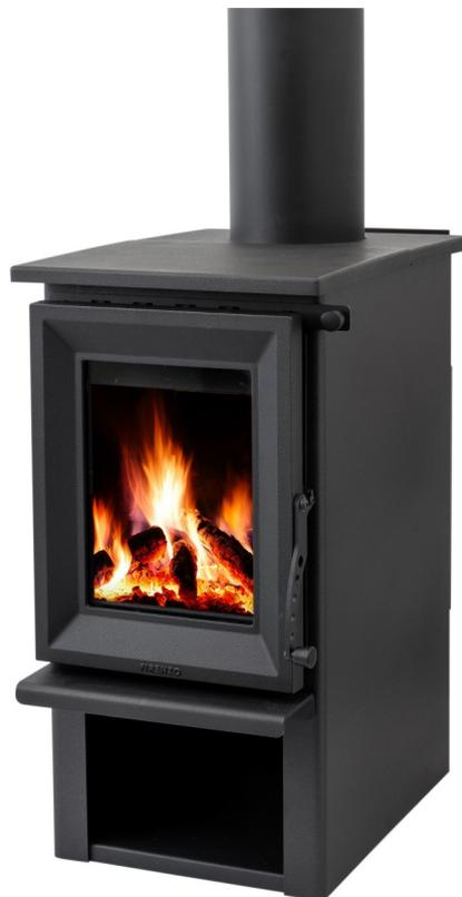
The Stella Woodfire can be installed on properties of less than 2 hectares of land and meets the ECAN standards with emissions of 0.5g per kg of fuel burned and 65% efficiency tested under AS/NZS 4012 and 4013:2014.
