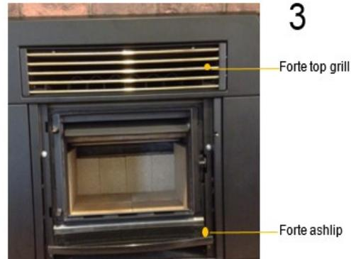
3. Refit the top grill. Remove the granite ashlip from the fascia box and fit below the door opening using the two locator screws at the bottom of the firebox (Screws for granite ashlip (5) see illustration 2). These two screws protrude by 5mm to enable the ashlip to be lifted up and over the
